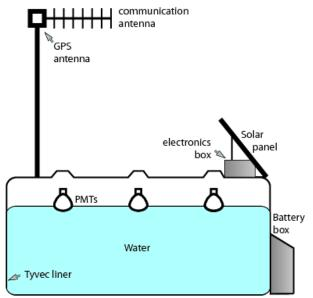
Each station filled with 12 tonnes of deionized water Passing charged particles produce Cherenkov light, detected by 3x(9" PMTs)Operational nearly 100% of the time 750 m array reduces lower energy limit from  $10^{18.5}$  eV to  $10^{17.5}$  eV
